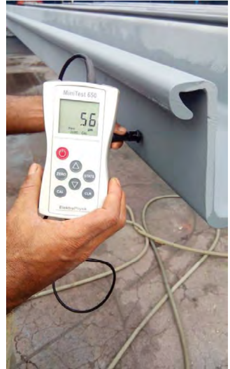
Dry Film Thickness (DFT) of the Corrosion Protection System
